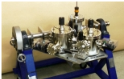
Figure 7. Ultra High Vacuum double monochromator, Model 234/302D
