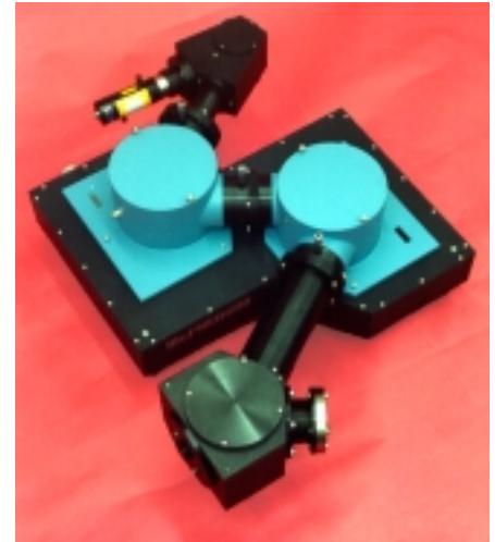
Figure 6. Dedicated vacuum UV double spectrometer, Model 234/302D
